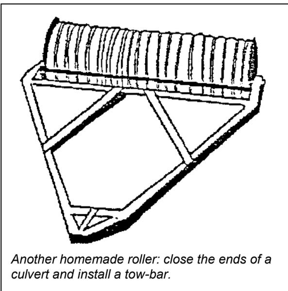
*Another homemade roller: close the ends of a culvert and install a tow-bar.*
