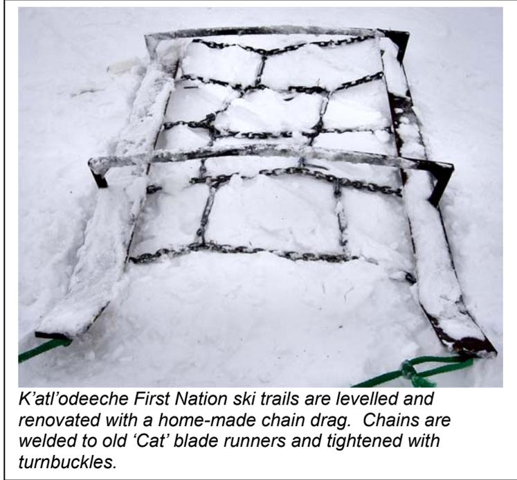
*K'atl'odeeche First Nation ski trails are levelled and renovated with a home-made chain drag. Chains are welded to old 'Cat' blade runners and tightened with turnbuckles.*
