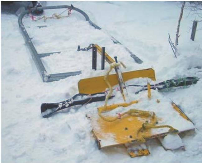
*One Pass Grooming: the Norman Wells Ski Club groomer drags a 'bed-frame' leveller and track-setter in tandem. The snowmobile does the packing.*
